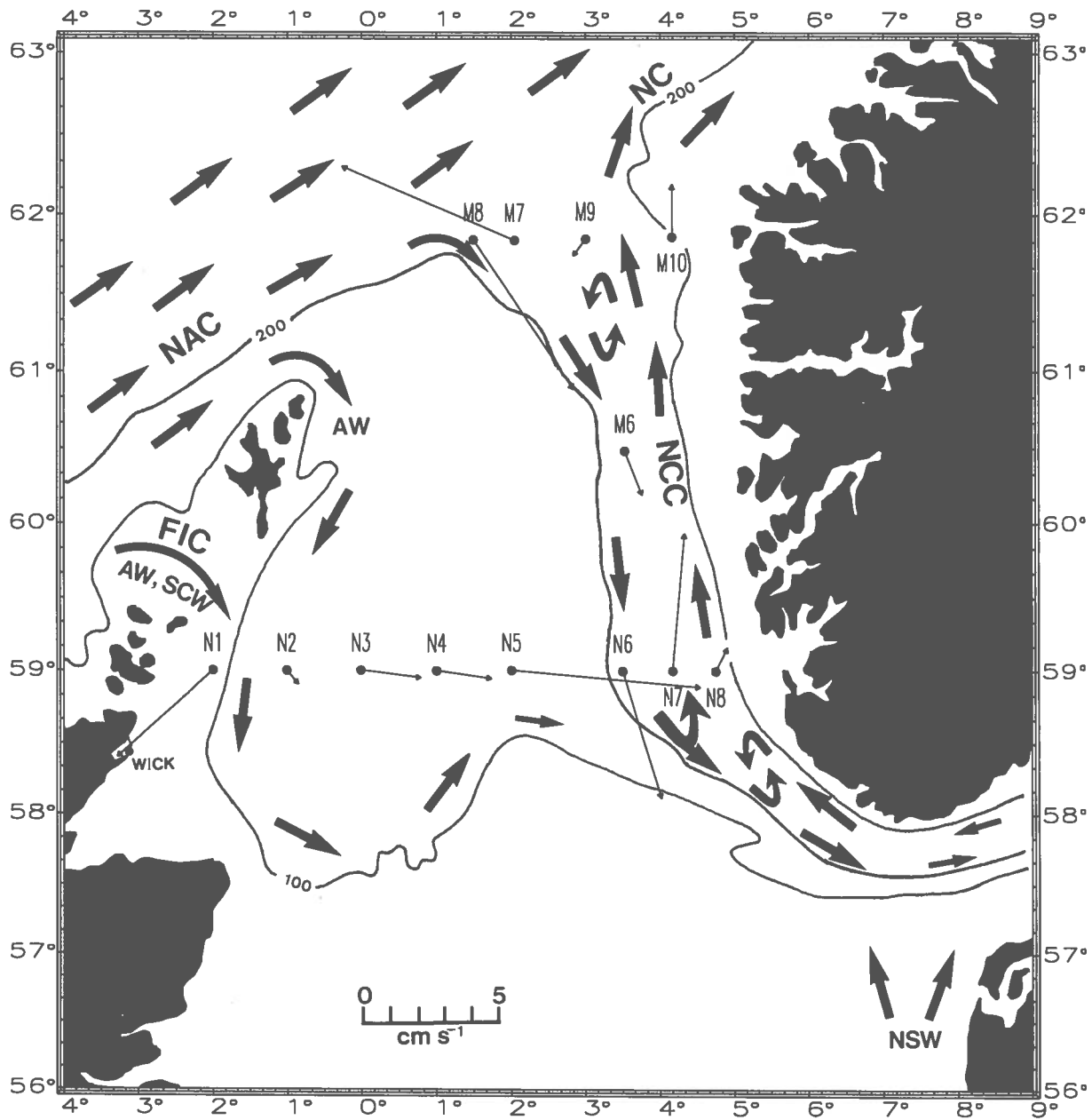
Fig. 1 Mooring positions and vertically (>30 m) averaged low-passed mean current vectors. The large scale circulation pattern is schematically outlined. NAC = North Atlantic Current, NC = Norwegian Current, NCC = Norwegian Coastal Current, FIC = Fair Isle Current. AW = Atlantic Water, SCW = Scottish Coastal Water.
