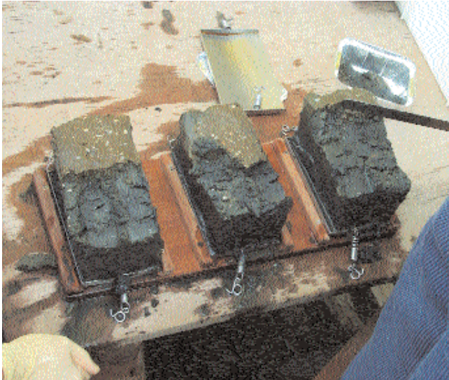
Sedimentproben aus Kastengreifer Sediment samples from box corer
