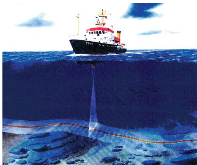
Fächerlot-Prinzip · Working principle of multi-beam echo system
