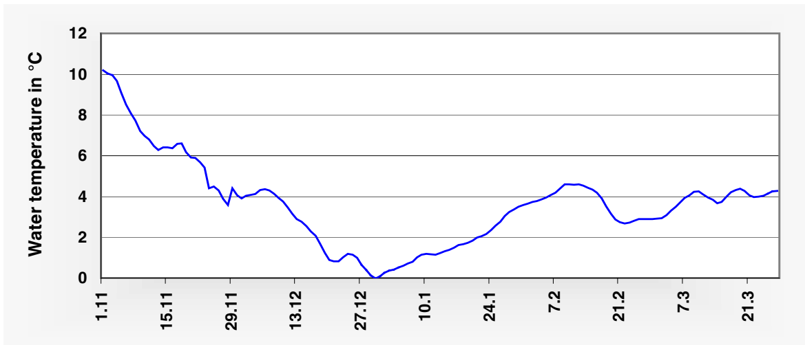
Figure 8.2. Running 5-day means of water temperature (at 3 m depth) in Koserow in the winter of 2001/02
